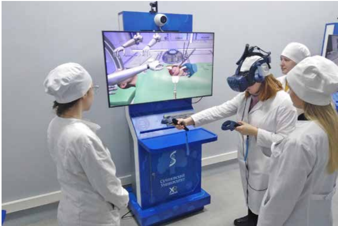
Figure 4. Work in a virtual operating room during the first stage of gastric resection surgery
